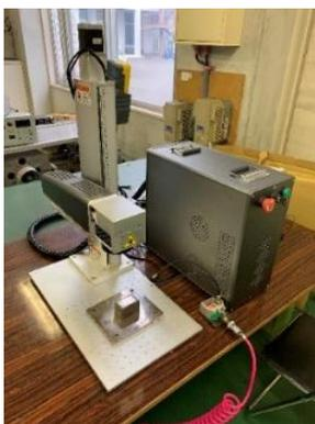
Fig.2 Pulse fiber laser.
