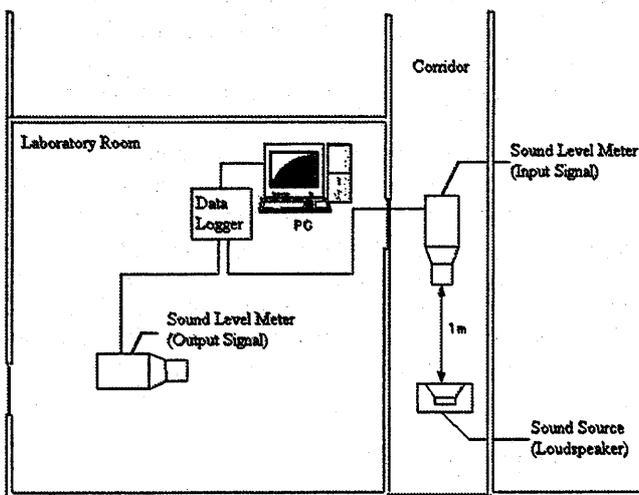
Fig.3 Arrangement of experimental apparatus.
