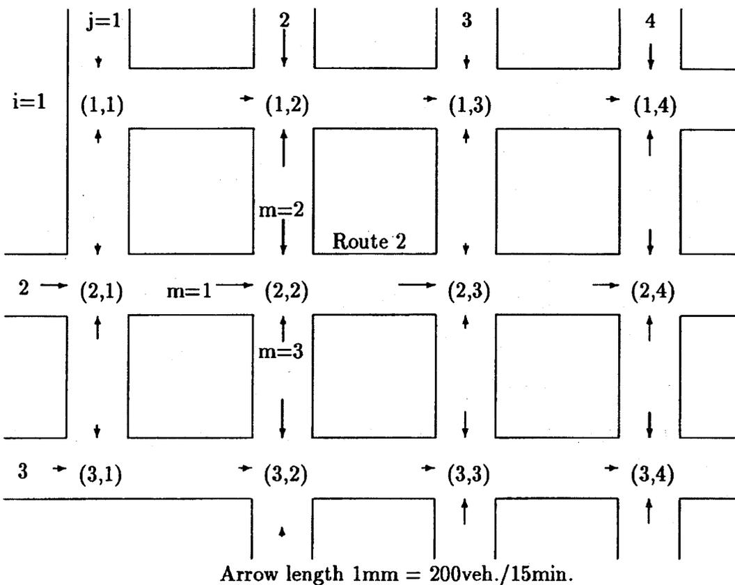
Fig. 9. Capacity at each signalized intersection (8:00-8:15).
