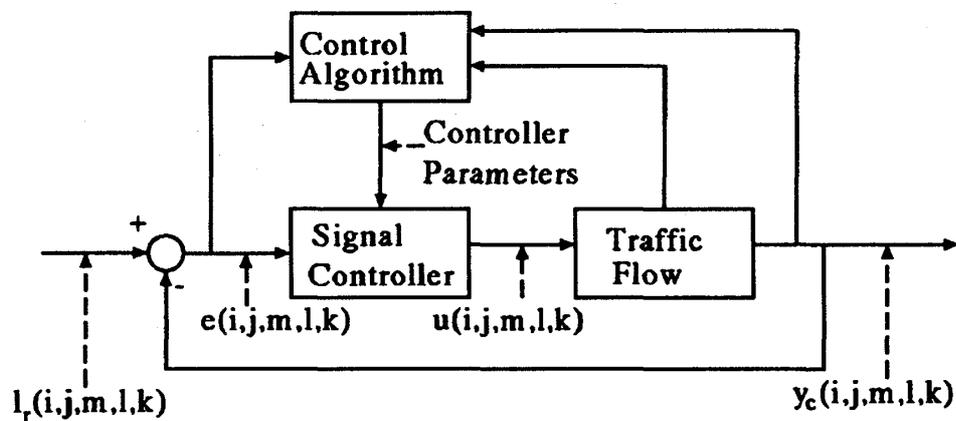
Fig.3. Signal control system.
