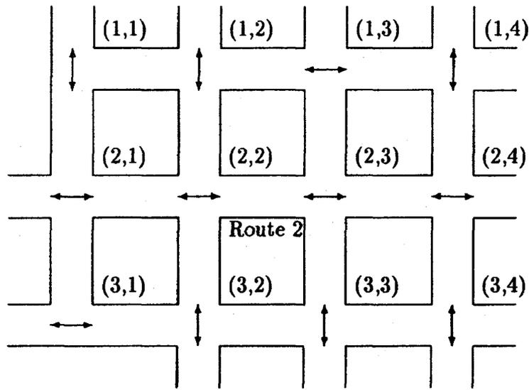
Fig.11. Priority directions of green time at each signalized intersection.
