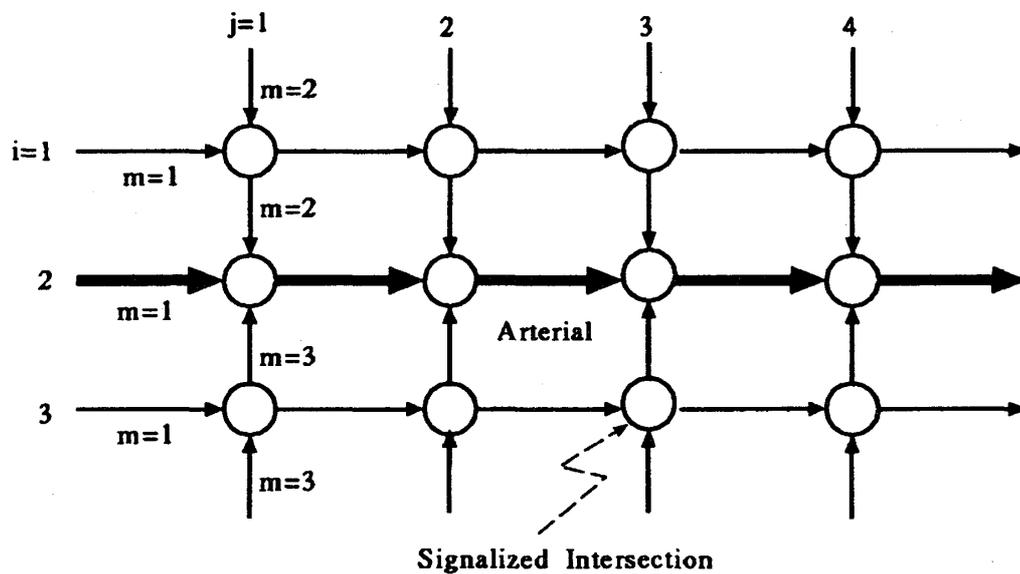
Fig.2. One-way traffic network consisting of a rectangular grid of intersecting streets.
