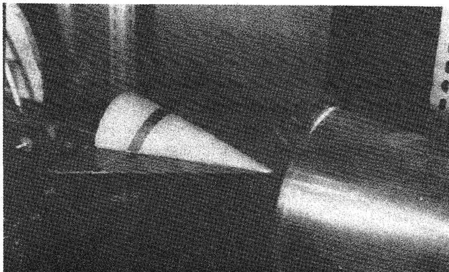
Fig.10 Test section including half cone body with delta wing.
