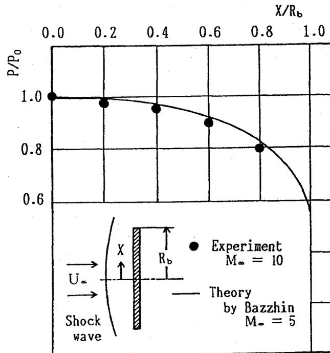
Fig.9 Pressure distribution on surface of flat plate.
