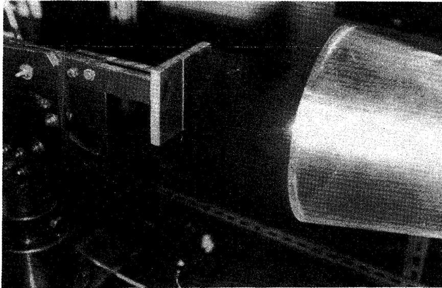
Fig.8 Test section including flat plate placed perpendicularly to hypersonic flow.
