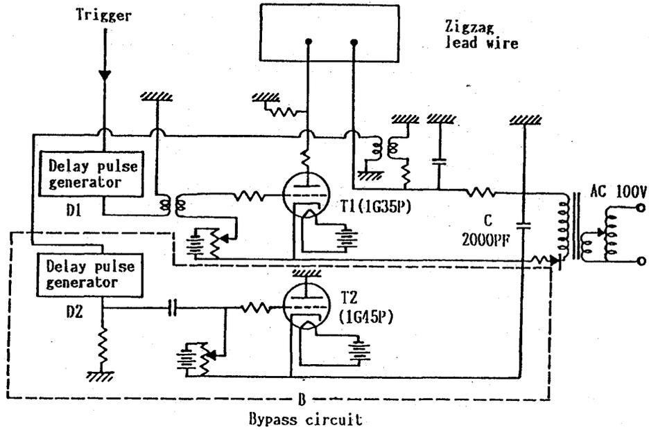
Fig.2 Electric circuit.
