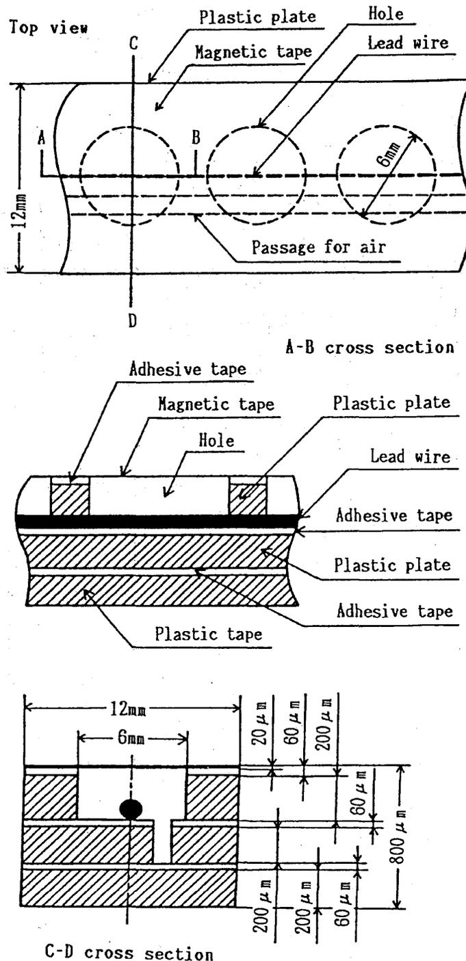
Fig.5 Pressure transducers designed and used in these experiments.
