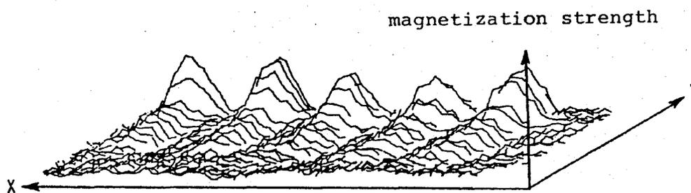
Fig.6 Example of distribution of magnetization strength on surface of magnetic tape.
