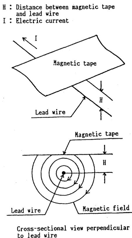
Fig.1 Illustration of visualizing Principle.
