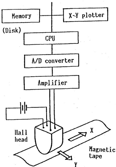
Fig.3 Measuring system of magnetization strength of tape.
