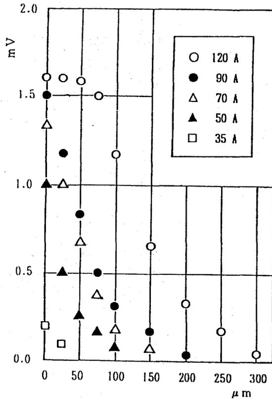
Fig.4 Relation between output Voltage and distance of lead wire and the magnetic tape under parameter of electric current in lead wire.
