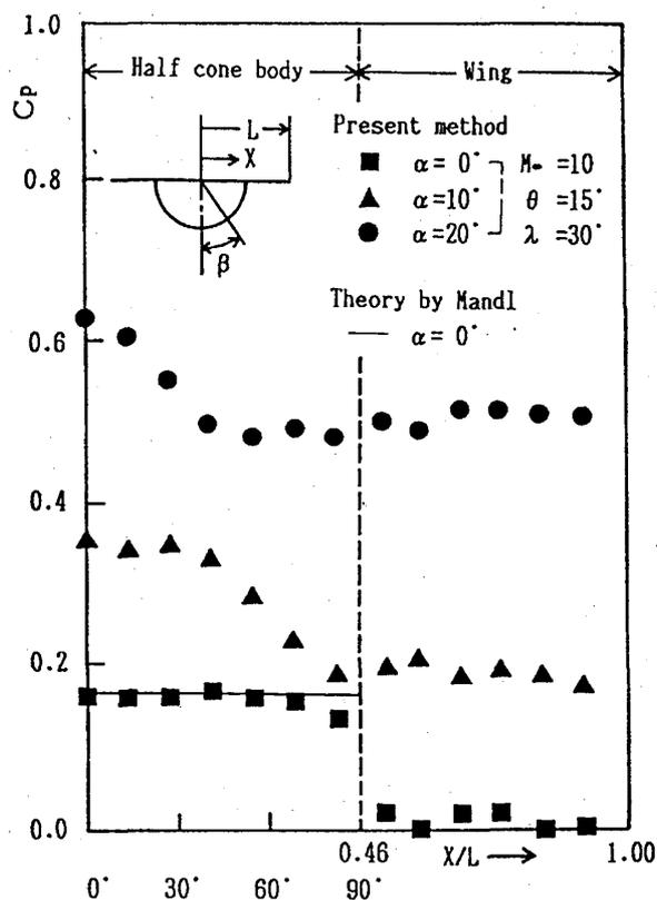
Fig.11 Pressure distribution around half cone body with delta wing.
